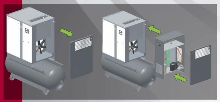
Compressor (C)  $\rightarrow$  Compressor mounted to a tank (CT)  $\rightarrow$  Addition of a integrated drier (CTD), to obtain a full station for the production, treatment and stocking of compressed air. All this is accomplished by simply removing a side panel from the compressor and reusing it as side closure for the drier.
