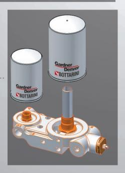
Improved fluid-mechanical efficiency is ensured by a new verticaldesign suction valve. Intake-air flows through a straight-line path, which guarantees lower load loss. ON/OFF operation and unloading is controlled via a solenoid valve.
